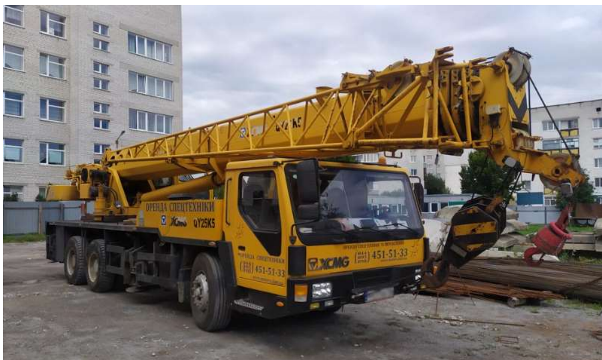
Picture 3.7 – XCMG QY25K5 Truck Crane
